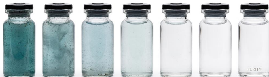
Figure 2. Visual progression of the photocatalytic decolorization of the methylene blue solution under irradiation, recorded at 0, 5, 15, 30, 60, 90 and 180 minutes.
